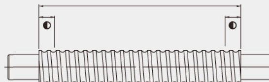
Fig 4.8 The heat treatment range of the ballscrew spindle
